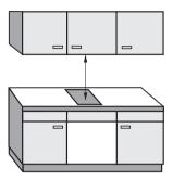
The minimum safety distance given by the hood manufacturer must be maintained between the combiset and the hood above it. See the installation instructions of the hood for these safety measurements.
